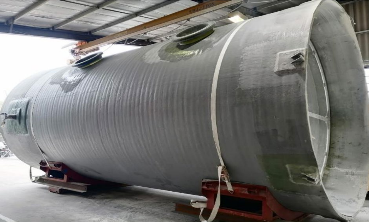
First Ion Exchange cylinder winding complete
